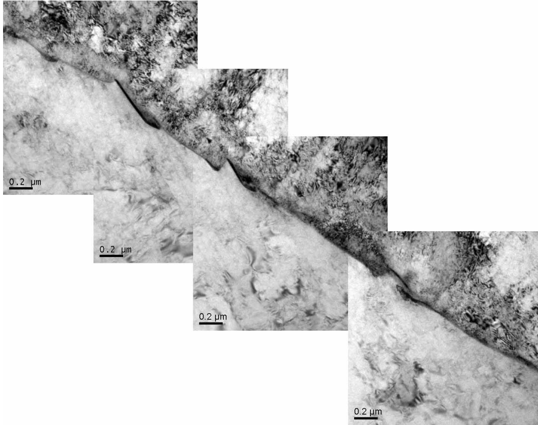
Figure 2: Chromium borides on a grain boundary in tube B.
