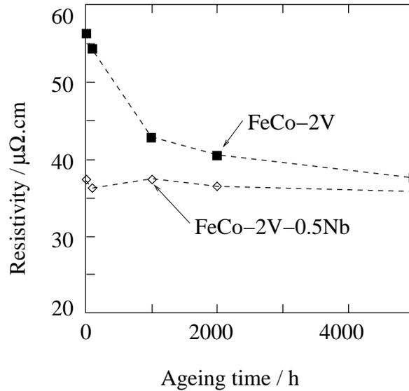
Figure 45: The resistivity of H50 and H50HS as a function of ageing at 550 °C, after [35].
