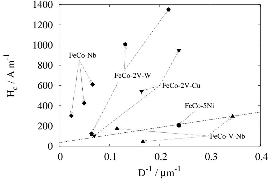
Figure 26: Coercivity of a variety of FeCo based alloys as a function of their grain size. FeCoV-Cu, FeCoV-W and FeCo-Ni from [19], FeCo2V-.3Nb from [32].
