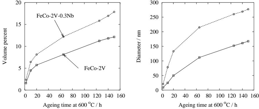
Figure 6: Volume percent and diameter of precipitates during ageing of FeCo-2V and FeCo-2V-0.3Nb according to Yu *et al.* [31].
