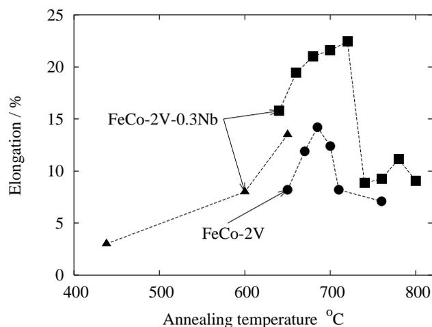
Figure 44: The ductility of FeCo-2V and FeCo-2V-0.3Nb alloys as a function of annealing temperature. All treatments 1 h for FeCo-2V-0.3Nb except at 438 °C (5 h), 2h for FeCo-2V. Lower temperature data for FeCo-2V-0.3Nb from [65], higher temperature from [93], data for FeCo-2V from [59].
