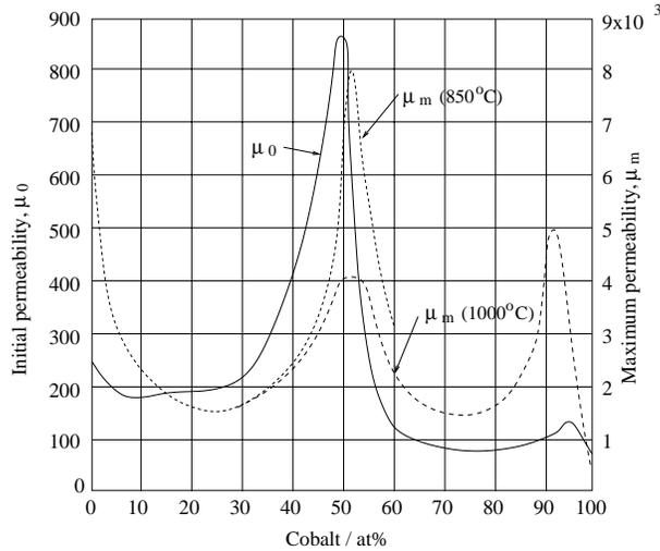
Figure 22: Initial and maximum permeability for Fe-Co alloys, the annealing temperature influences strongly the maximum permeability, in this case most likely because 1000 °C lies in the two-phase region. After [67].
