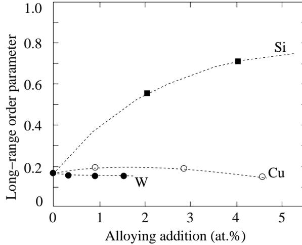
Figure 19: The variation of long-range order parameter for 2.5 mm strips of various compositions, quenched from 850 °C. After [19].
