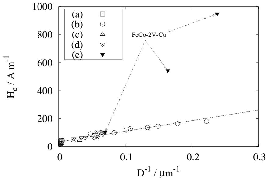
Figure 25: Coercivity of a variety of FeCo based alloys as a function of their grain size. (a) Stanley, 1950, for FeCo-2V [79] (b) Yu *et al.*, 2000, for FeCo-2V [31], (c) Major *et al.*, 1988, for FeCo-0.2Ta [91] (d) Orrock, 1986, for FeCo-2V [19], all are annealed and single-phase. FeCo-V-Cu from [19].
