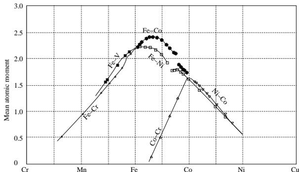
Figure 21: The Slater-Pauling curve showing the mean atomic moment for a variety of binary alloys as a function of their composition, after [67].
