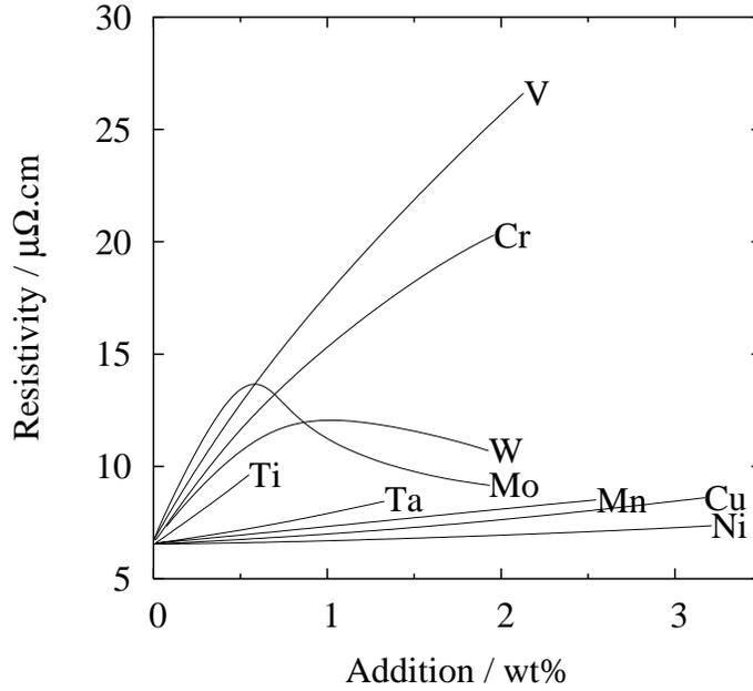
Figure 29: The influence of various addition on the resistivity of FeCo alloys. After [67].
