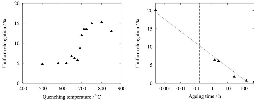
Figure 41: Uniform elongation at room temperature of Fe-48Co-2V samples quenched in iced brine after annealing 30 min at various temperatures, after [75].
