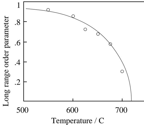
Figure 13: The long range order parameter as a function of temperature in FeCo, after [75].
