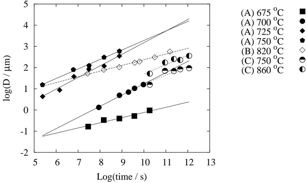
Figure 9: The grain size as a function of time during annealing at varying temperatures following deformation. (A) FeCo-2V, drawn, area reduction 75% [57], (B) FeCo-2V-.05Nb, cold-rolled, thickness reduction presumed 90% [58], (C) FeCo, cold-rolled, thickness reduction 82% [55].
