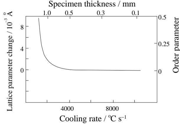
Figure 11: The lattice parameter change caused by ordering as a function of the cooling rate, in equiatomic FeCo, and FeCo-2.5V. The ordering reaction can be avoided with cooling rates greater than  $\sim 4000$  °C/s. After [68].
