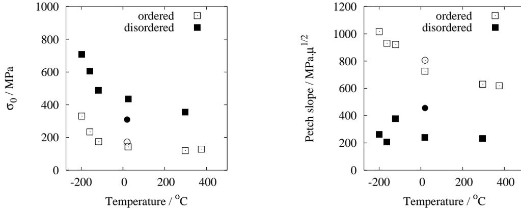
Figure 39: The Hall-Petch parameters  $\sigma_0$  and  $k$  as measured by Jordan and Stoloff for FeCo-2V at different temperatures [98]. Superimposed (circles) are the results of Zhao and Baker for FeCo *et al.* [91] at room temperature.
