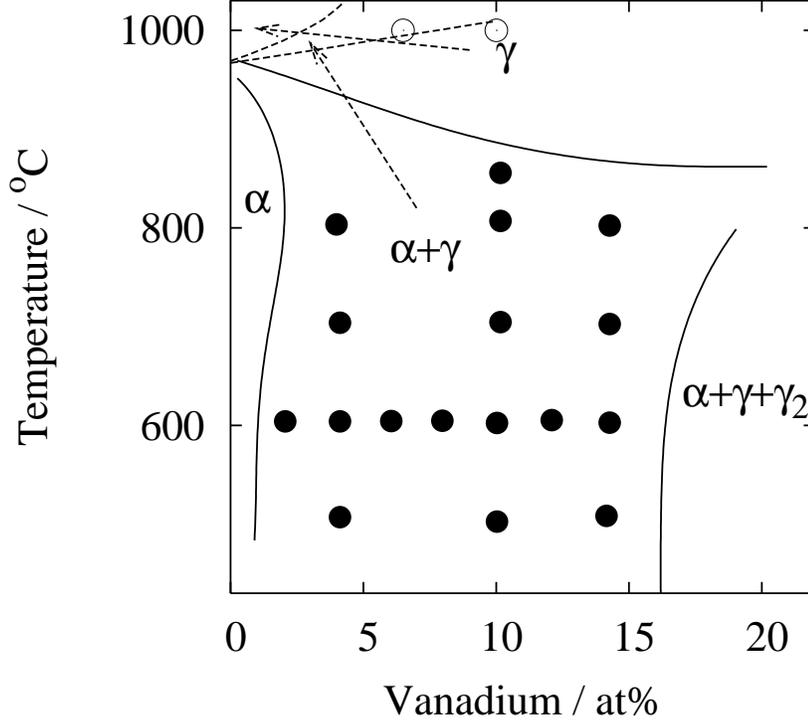
Figure 2: Isopleth section at 52 at% Co for the FeCoV system. Dotted lines indicate the calculation made using MT-DATA and the SGTE solution database, solid lines and data point are from Koster *et al.* [21, 22];  $\circ$  are points identified as single-phased regions and  $\bullet$  as two-phases regions.
