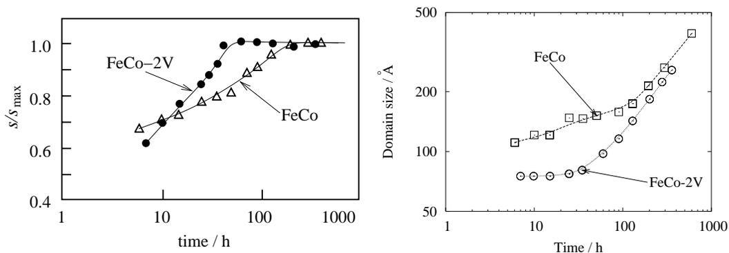
Figure 15: Isothermal ordering kinetics at 440 °C for FeCo and FeCo-2V quenched from 780 °C. After Eymery *et al.* [80]. Isothermal domain growth in same conditions, after Grobras *et al.* [76].
