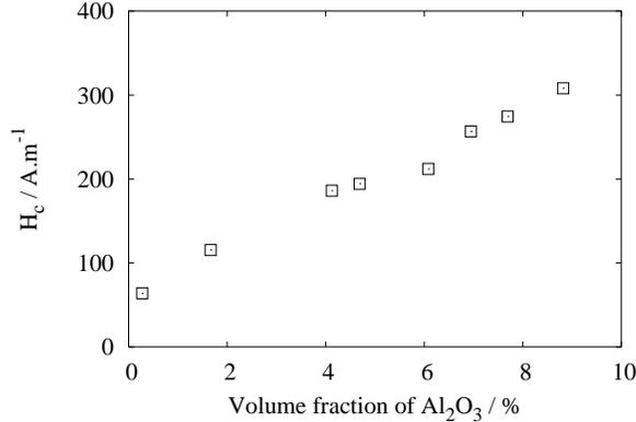
Figure 27: Coercivity of a W-fibres reinforced FeCo, with addition of  $\text{Al}_2\text{O}_3$  particles in increasing volume fraction, after [31].
