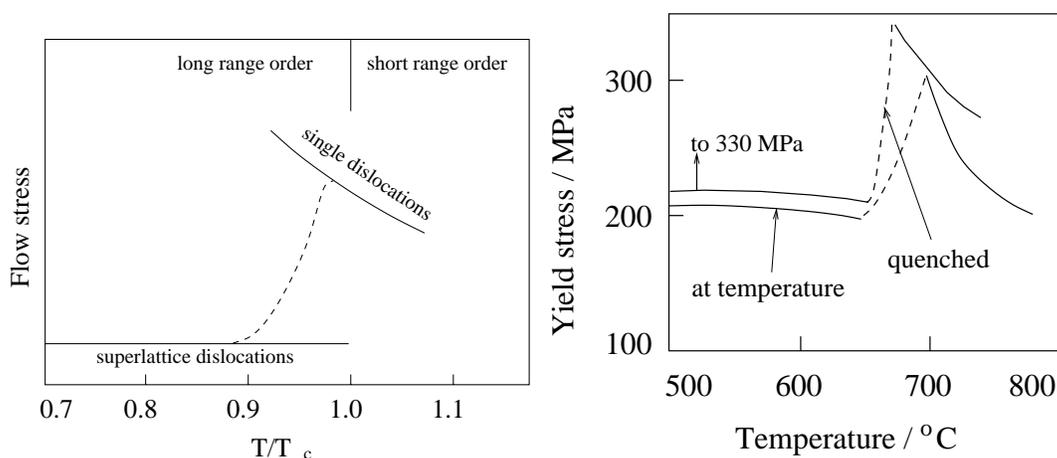
Figure 32: Illustration of the mechanism proposed by Stoloff and Davies to explain the influence of order/disorder (and of temperature through order/disorder) on the yield strength of FeCo based alloys, after [75]. Predictions by Moine *et al.*, for yield strength measured at indicated temperature and after quenching from the indicated temperature, after [97]. Note that the curve for quench temperature has been shifted to lower values for easier comparison.
