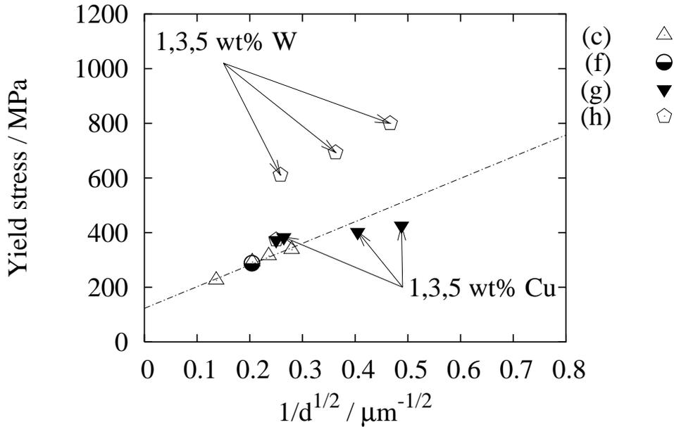
Figure 37: The strength of a variety of FeCo based alloys in well annealed, ordered condition. (c) as for figure 36; (f) FeCo-2V held 1 h at 825 °C then 24 h at 550 °C, 48 h at 500 °C the slow cooled to room temperature [82];(g) FeCo-2V-Cu held 2 h at 850 °C then slowly cooled at 120 °C/h [19]; FeCo-2V-W, similar heat-treatment [19].
