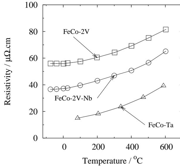
Figure 30: The resistivity of FeCo-V, FeCo-V-Nb and FeCo-Ta as a function of temperature, after [35] and [94].
