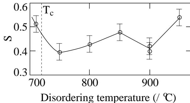
Figure 20: The degree of order achieved after 500 s at 450 °C in a 48.4Fe-49.8Co-1.8V wt%, as a function of the prior ‘disordering’ temperature.
