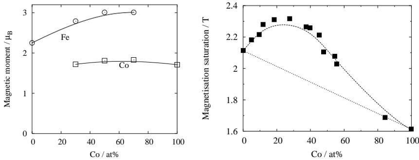
Figure 23: The magnetic moments of Fe and Co on binary alloys of different compositions, after [87]. The saturation magnetisation of  $\text{Fe}_{1-x}\text{Co}_x$  alloys as a function of composition. The straight line is that for an unmilled mixture of pure elements. The formation of a solution is accompanied by an increase in the saturation magnetisation. After [88].
