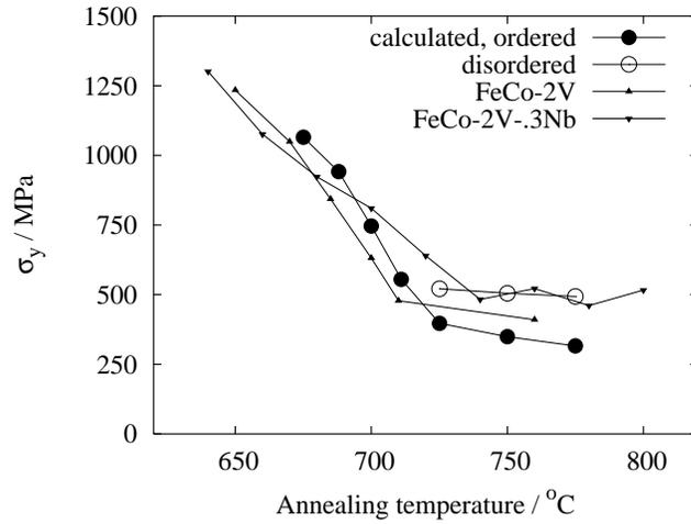
Figure 40: The strength of FeCo-V and FeCo-V-Nb alloys, as measured by Thornburg [59] and Hailer [93] respectively. Calculation for FeCo-2V using the grain sizes reported by Davies and Stoloff [57], assuming in a first instance, that all samples are ordered (filled circles), and in a second study, that samples cooled from above  $T_c$  are disordered (empty circles).
