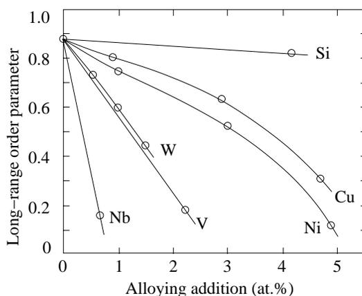
Figure 16: The ordering parameter of binary and ternary FeCo alloys as a function of elemental additions, after quenching into ice brine from 730 °C. After [19, 81].
