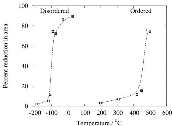
Figure 42: The ductility of ordered and disordered FeCo-2V as a function of temperature, after [99].
