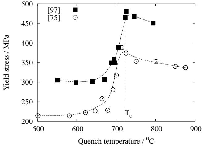
Figure 31: The 0.1% yield stress for FeCo-2V samples quenched from different temperatures so as to produce different degree of long range order, after [75] and [97].
