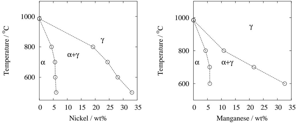
Figure 8: The influence of Ni and Mn on the  $\alpha/\alpha+\gamma$  and  $\alpha+\gamma/\gamma$  boundaries. FeCo-Ni constructed from the isotherm sections in [46]. FeCo-Mn from isotherm sections in [49]. It should be noted that these isotherms are largely extrapolated if not guessed in this region.
