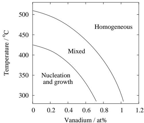
Figure 17: The ordering mechanism of FeCo-V alloys as a function of temperature and vanadium content, for samples quenched from 800 °C, after [77].
