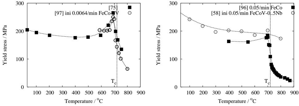
Figure 33: Variation of yield strength with temperature (a) for FeCo-2V [75,97] showing significant increase of strength as the temperature increases to the critical temperature for ordering, (b) for FeCo [96] and FeCo-2V-0.03Nb [58] showing little increase of strength before the  $T_c$ .
