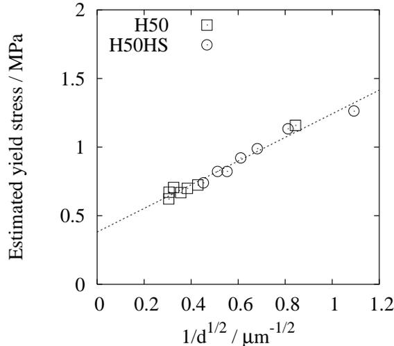
Figure 35: The grain size dependence of FeCo-2V (H50) and FeCo-2V-Nb (H50HS) showing a unique Hall-Petch line regardless of the fact that the latter alloy contains second-phase precipitates, after [33].
