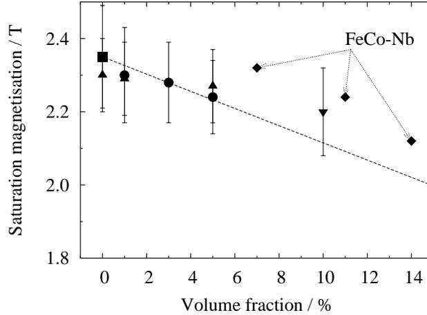
Figure 24: The saturation of a variety of FeCo based alloy as a function of the volume fraction of paramagnetic second phase, after [19, 24]
