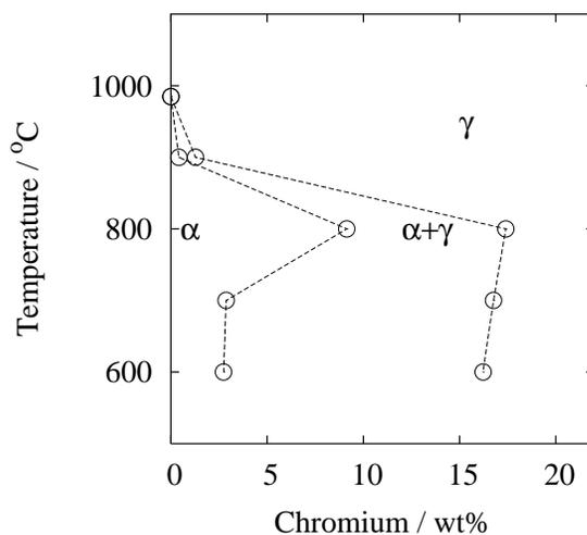
Figure 7: The influence of Cr on the  $\alpha/\alpha + \gamma$  and  $\alpha + \gamma/\gamma$  boundaries. Constructed from the isotherm section in [46]. These isotherms are largely extrapolated if not guessed in this region.
