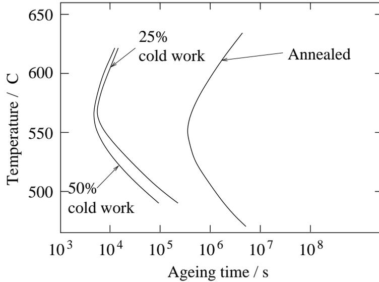
Figure 5: TTP diagram for intragranular  $\gamma_2$  formation in FeCo-2%V, after Ashby *et al.* [10].
