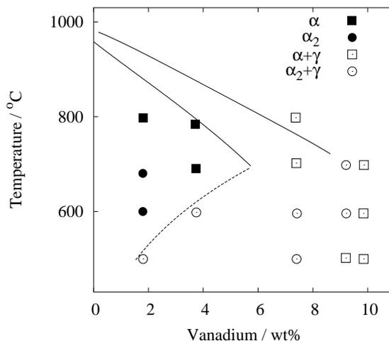
Figure 3: Isopleth section at 52% Co in FeCo-V system, after Martin and Geisler [16]. Solid lines indicate boundaries determined by thermal analyses, phases are otherwise identified by X-ray diffraction.
