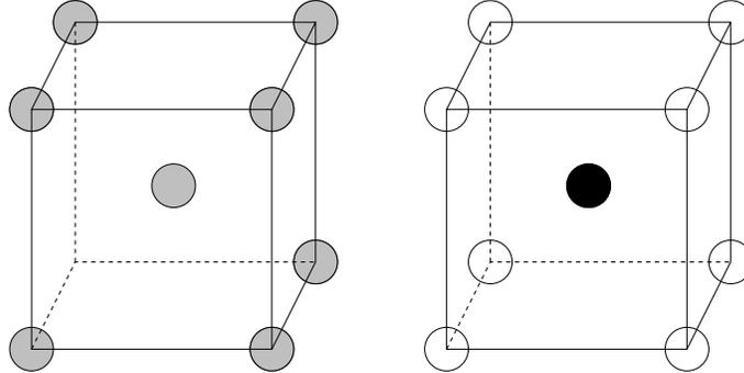
Figure 10: b.c.c. and ordered B2 structure.
