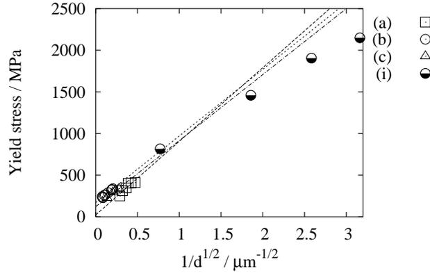
Figure 38: The strength of FeCo-2V-0.5Nb with sub-micron grain size. Series (a) to (c) as in figure 36 and 37; (i) data from Duckham *et al.* [65].
