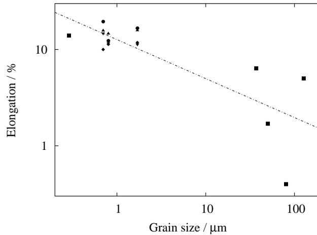
Figure 43: The ductility of FeCo-2V and FeCo2V-Ni alloys as a function of their grain size, using data from [65,75,113].
