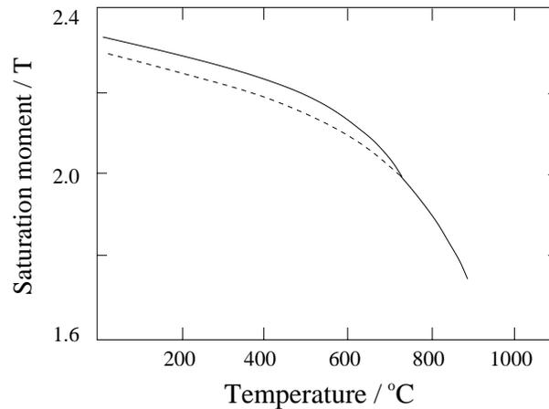
Figure 12: The variation of the saturation magnetisation as a function of temperature, after [68].
