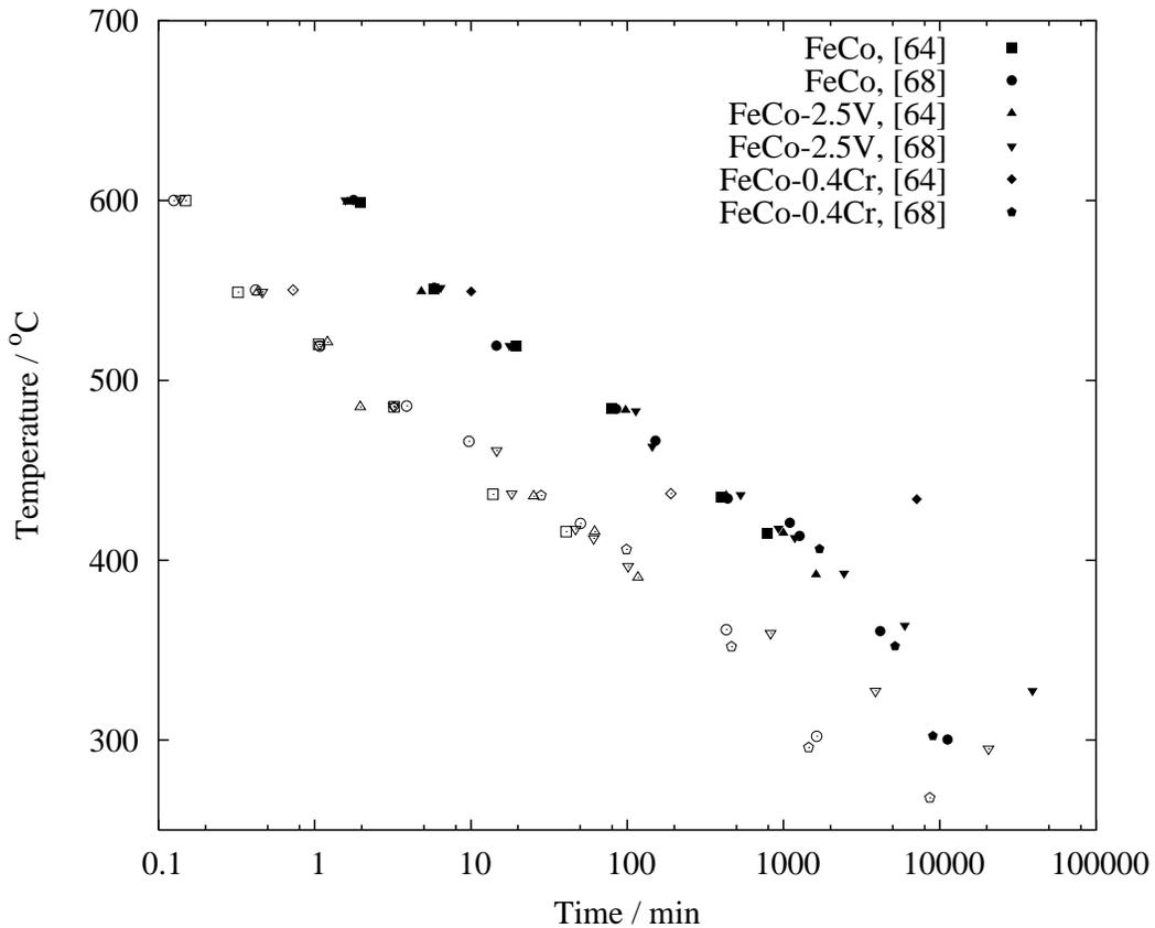
Figure 14: The times to reach  $S/S_{max}=0.5$  (empty symbols) and  $S/S_{max}=0.95$  (full symbols) in FeCo based alloys with different additions, after quench in iced brine from 810 °C. After [64, 68].
