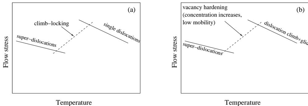
Figure 34: Schematic illustration of the mechanism proposed by Morris [102] (a) and George and Baker [107] to explain the peak strength of FeAl at intermediate temperatures.
