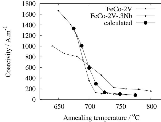
Figure 28: Coercivity of FeCo-2V [59] and FeCo-2V-0.3Nb [93] after annealing at different temperature, for 1 h in the case of FeCo-2V-0.3Nb, 2 h for the FeCo-2V alloy. Exact measurement conditions are not indicated in [59]; for FeCo-2V-0.3Nb [93], coercivity was measured with maximum applied field of 1.59 T, at 60 Hz. This is compared with calculations for FeCo-2V using equation 10 and the grain sizes reported by Davies and Stoloff [57].
