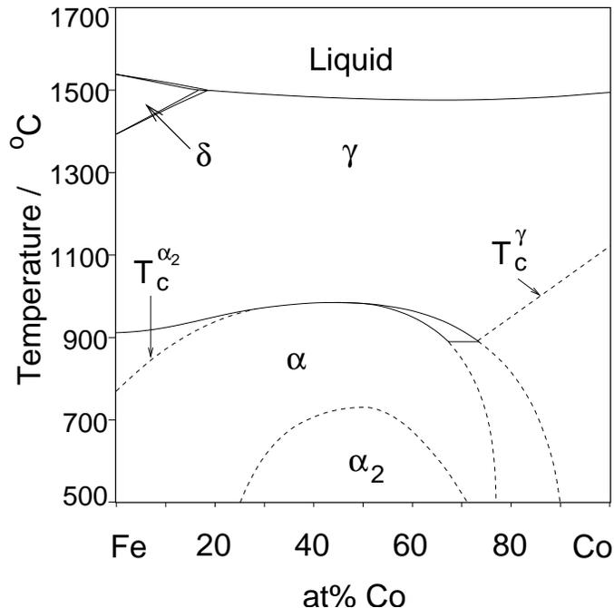
Figure 1: The Fe-Co binary diagram as given in [5].  $T_c$  denotes the Curie temperature.
